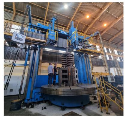
We have now modernised the machine and installed it on a heavy-duty foundation in our heavy bay.
