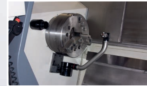
Manual tool measuring arm
