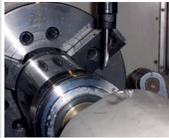
Tool turret for driven tools with integrated Y-axis
