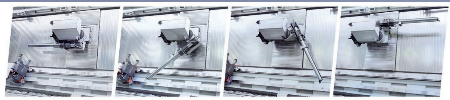
Special boring bar attachment for deep boring operation. The unit is designed for boring bar 120 mm in diameter. The boring bar is mounted on swivel holder that lets the bar be put on parking position without disassembling.
