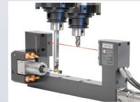
Combined tool setting system: non-contact measurement of rotating tools with laser and touch probe for static tools
